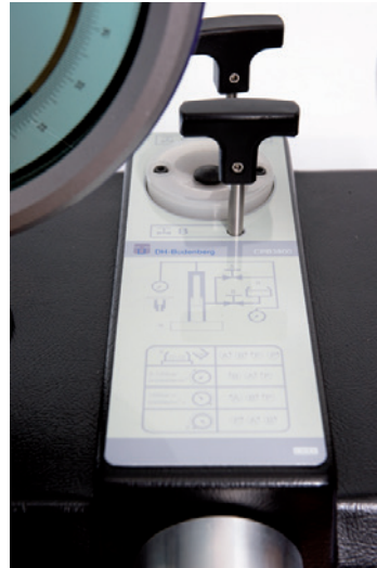
Control schematic on the CPB3800HP instrument base
